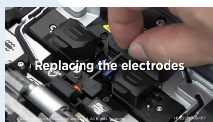
Replacing the electrodes
